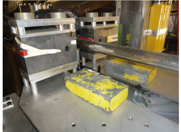
Fig. 4: Collimators in situ . Photo taken during final alignment, some survey equipment pictured atop collimators.
