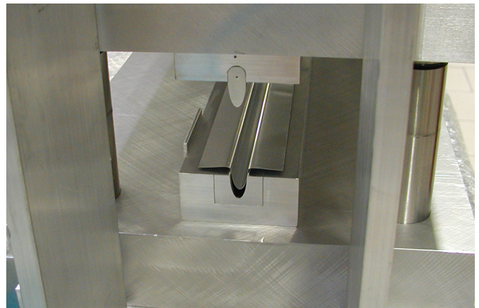
Figure 4: The target cell foil in the pneumatic press before (a) and after (b) shaping
