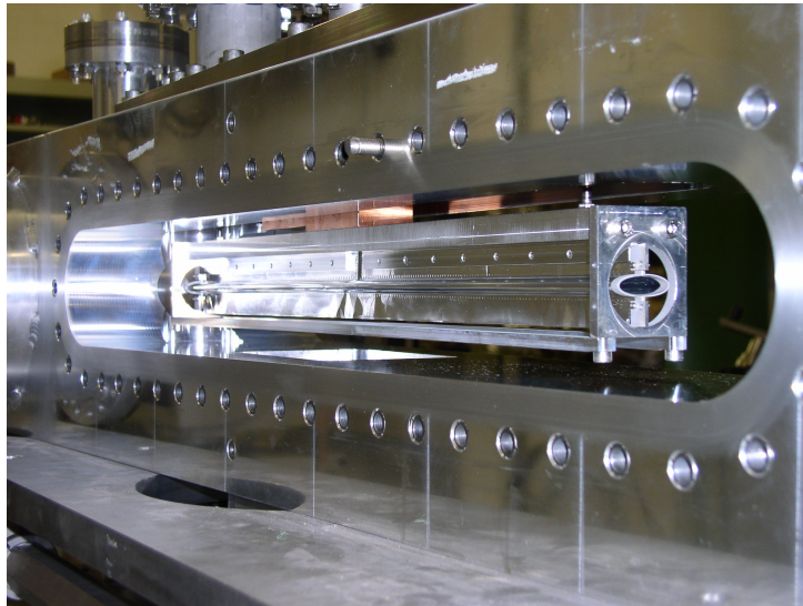
Fig. 3: Photograph of one of the OLYMPUS target cells mounted inside the scattering chamber.
