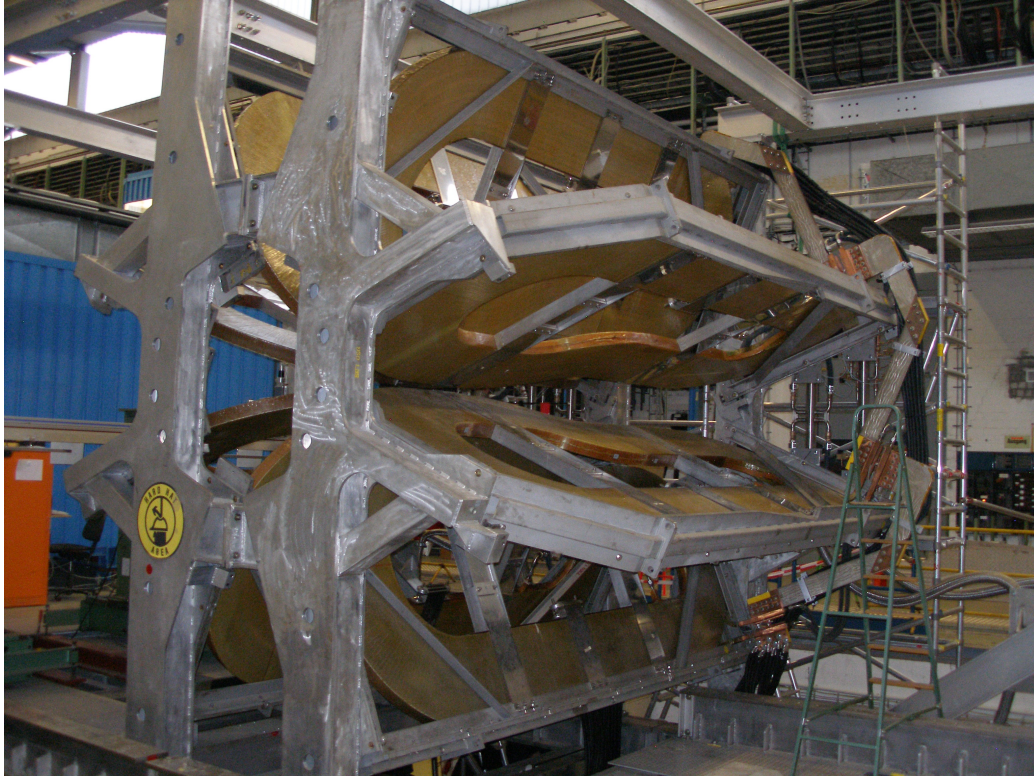
Fig. 10: The toroid magnet assembled at DESY before the subdetectors were installed
