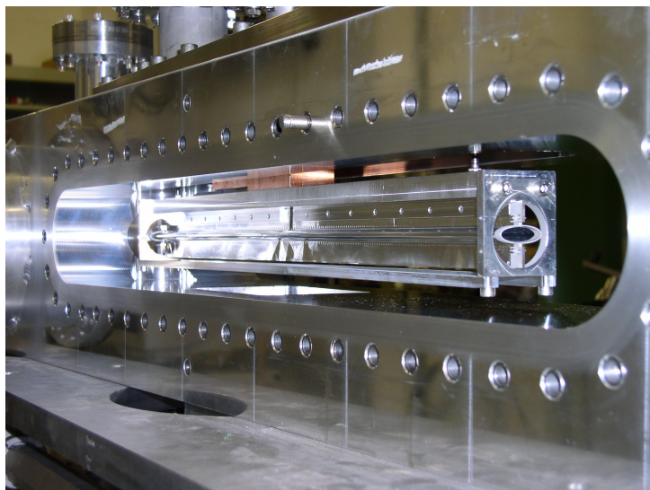
Figure 1: Photograph of one of the OLYMPUS target cells mounted inside the scattering chamber.
