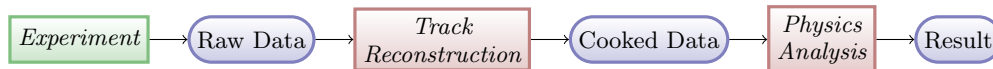
FIG. 1. The data analysis chain: rectangular red nodes represent a software process, while the rounded blue nodes represent some type of data object.
