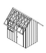
Cut two 1x4s to run along the trusses at the top of the roof. Use 2" screws to screw into roof truss. Cut two 2 x 4 eaves about 8' 1 1/2" to cover the ends of the trusses. Use 3 1/2" screws to attach.
