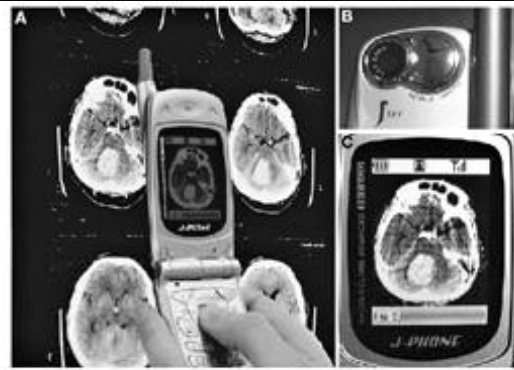
FIGURE 1. A , CT scan of a cerebellar hemorrhage being photographed by a mobile phone with a digital camera. B , mobile phone as combined with a 110,000-pixel digital camera used to transfer the CT scan. C , CT scan as received via a mobile phone with a thin-film transistor liquid crystal display, which can display up to 65,536 colors.
