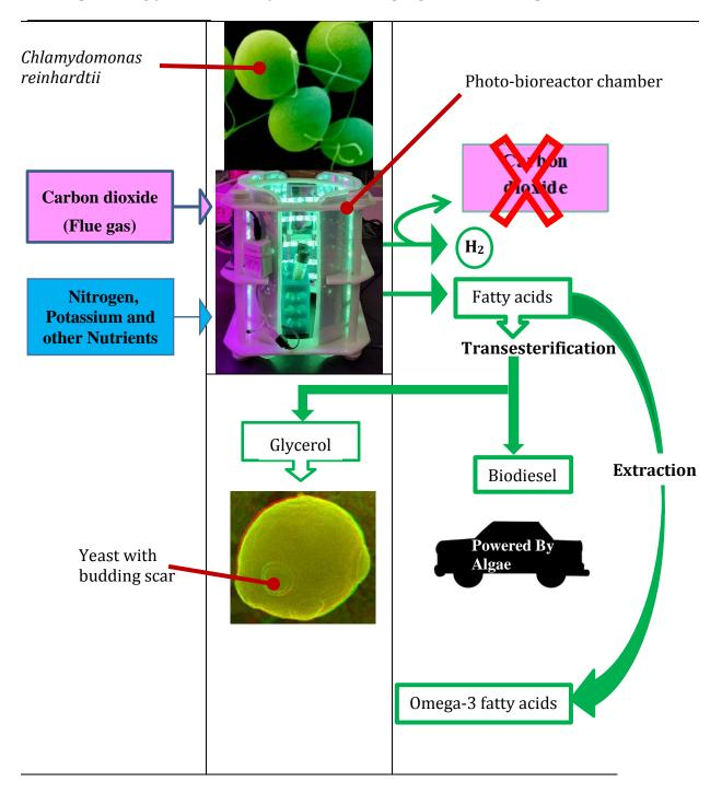
A yeast/microalgae platform will be set up this summer for the proposed research, and include the photobioreactor shown above (for the microalgae).
