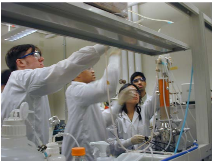
Team members set up their fluidized-bed reactor in the continuous mode (called “perfusion”) during a process for IgG production
