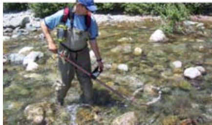
Juvenile steelhead implanted with transponder tags tracked using a portable antenna
